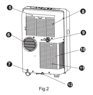
**Operation Panel (**) Horizontal Louvers 2 3 Caster **Carrying Handle** 4 (both sides) 5 Upper Air Filter (Behind the grille) 6 Air Outlet Power cord outlet 67 8 Air intake **Drain Outlet** 9 Air intake 1 Lower Air Filter (Behind the grille) 12 **Bottom Drain Plug**
